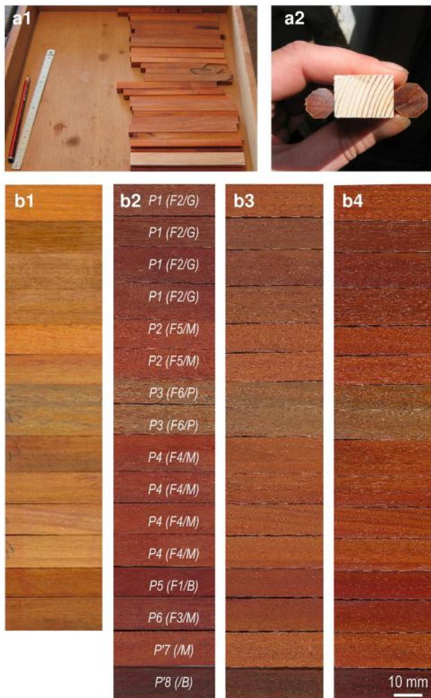
Figure 1: Studied sampling of pernambuco. (a) Specimens’ preparation, (b) appearance and history. (a1) Pre-cuts from uneven-shaped bow-making offcuts; (a2) semi-finished broken bow-sticks, glued to unused wood to allow machining (b1, b2) raw-cut (fine circular saw) surfaces (b1) freshly cut (b2) after 18 years ageing; the batch number (P1–P’8), “feeling rank” (F1–F6), and “quality grouping” (P: ‘Poor’, M: ‘Medium’, G: ‘Good’, B: ‘Better’) are indicated (b3) “refreshed” (sanded at grit #220) and (b4) polished (grit #4000) surfaces. Note: earlier images (b1) were obtained with a different optical scanner than later images (b2, b3 and b4, that were imaged with a single scanner).
